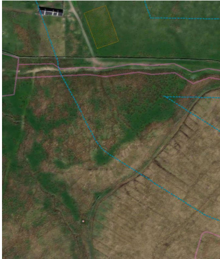
Figure 4.3: Aerial imagery showing the track marks from the existing track at Crockroy through to the Polmeurhill Plantation boundary (ILA area shown in blue and working areas in orange; access tracks not shown)
