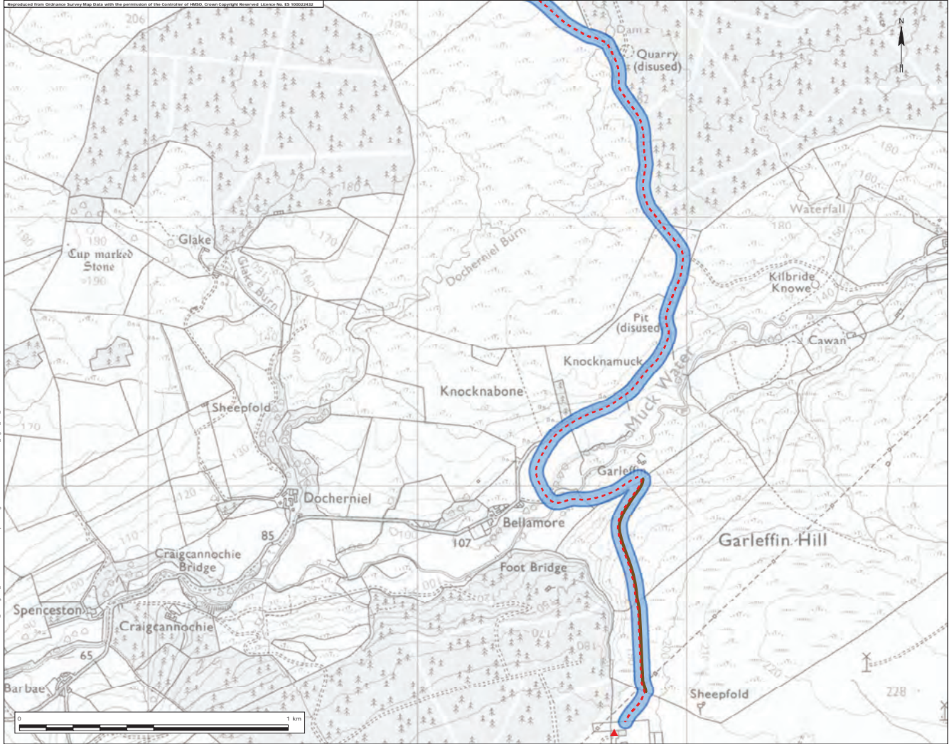
Figure 3.1d: Indicative Wood Pole Positions and Limits of Deviation (LoD)
