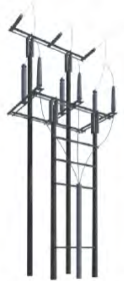
Component parts of 132kV 'Trident' design wood pole: Terminal (H pole)
