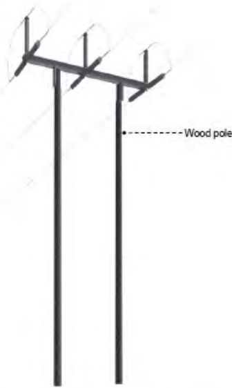
Component parts of 132kV 'Trident' design wood pole: Angle (H pole)
