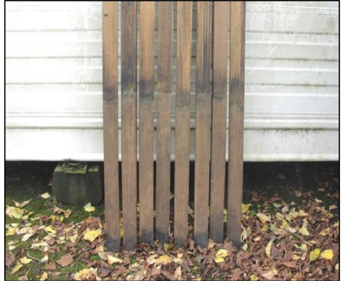
Tanasote treated unsleeved stakes at 48 months: no overt indications of decay noted on these stakes.
