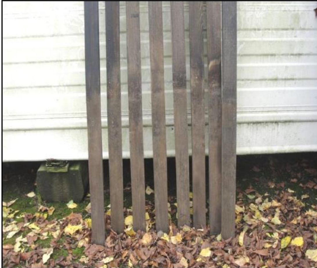
RVP treated unsleeved stakes at 48 months: no overt indications of decay were noted on these stakes.
