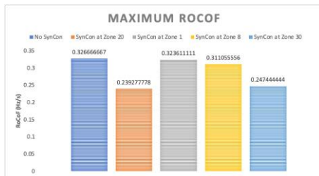
Figure 40 - RoCoF values for Scenario 3 (LoG in Zone 20) considering different SC locations.
