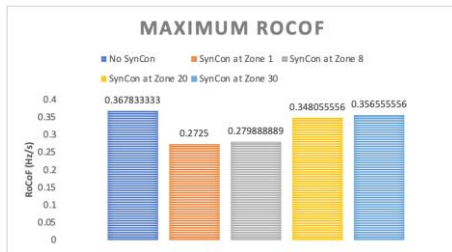
Figure 38 - RoCoF values for Scenario 1 (LoG in Zone 1) considering different SC locations.
