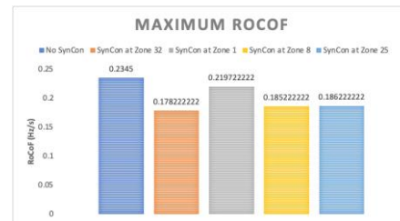
Figure 41 - RoCoF values for Scenario 4 (LoG in Zone 32) considering different SC locations.
