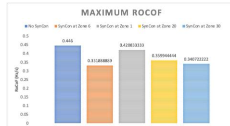
Figure 39 - RoCoF values for Scenario 2 (LoG in Zone 6) considering different SC locations.
