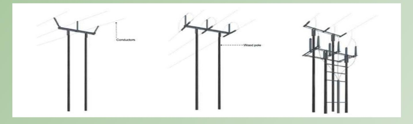
Trident wood poles are typically galvanised steelwork cross-arms supporting aluminium conductors on insulators. These are suitable for supporting single circuit lines operating at 132 kV. Wood poles are fabricated from pressure impregnated softwood, treated with a preservation to prevent damage to structural integrity.
