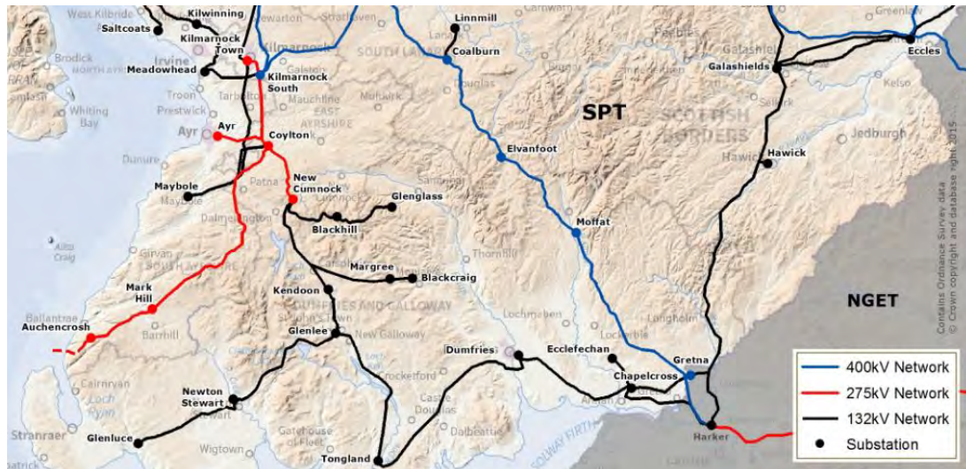
Figure 2.1 Electricity transmission system in south-west Scotland
