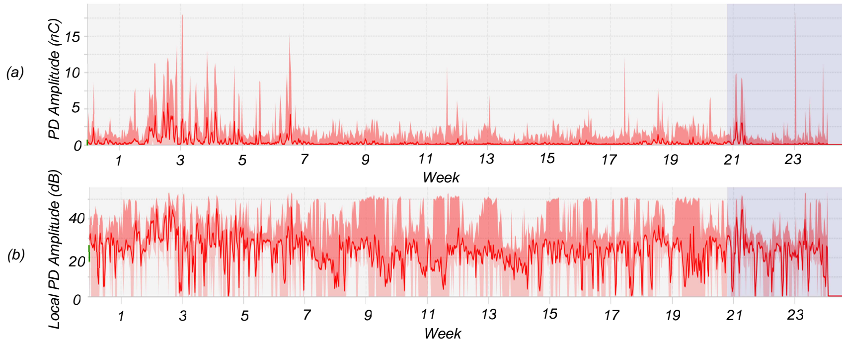
Figure 10. Raw time series sensor data showing PD amplitude from HFCTs and TEV sensors over a 21 week period (09/02/2017 – 13/07/2017).
