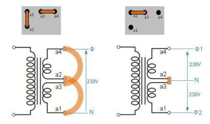
As the figures indicate, the 'conventional' link arrangement provides a single phase supply of 50kVA or 100kVA from a 50kVA or 100kVA transformer respectively. The split phase operation either provides a 50kVA (or 100kVA) two phase 480V supply or more commonly two 25kVA (or 50kVA) single phase supplies. It should be noted that winding arrangement indicated results in a phase angle difference of 180° for the two windings and therefore external paralleling the connections is not possible.
