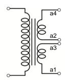
The method of achieving split phase operation will vary with manufacturer but a typical example is shown in the following figures. The left figure shows the link arrangement and resultant winding connections for a conventional LV single phase supply with the schematic on the right indicating the link arrangement and resultant winding connectivity for split phase operation.
