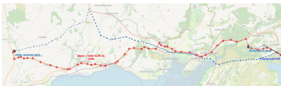
Figure 8. Proposed 132kV cable route and site location
