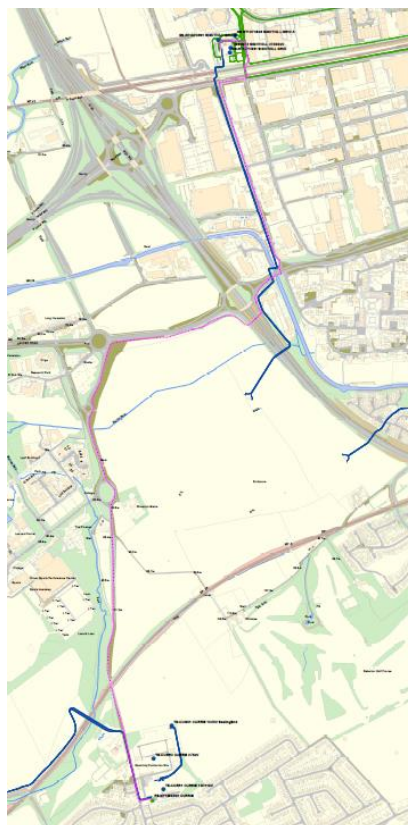
Figure 8. Proposed route for 33kV circuits from Sighthill GSP to Currie primary
