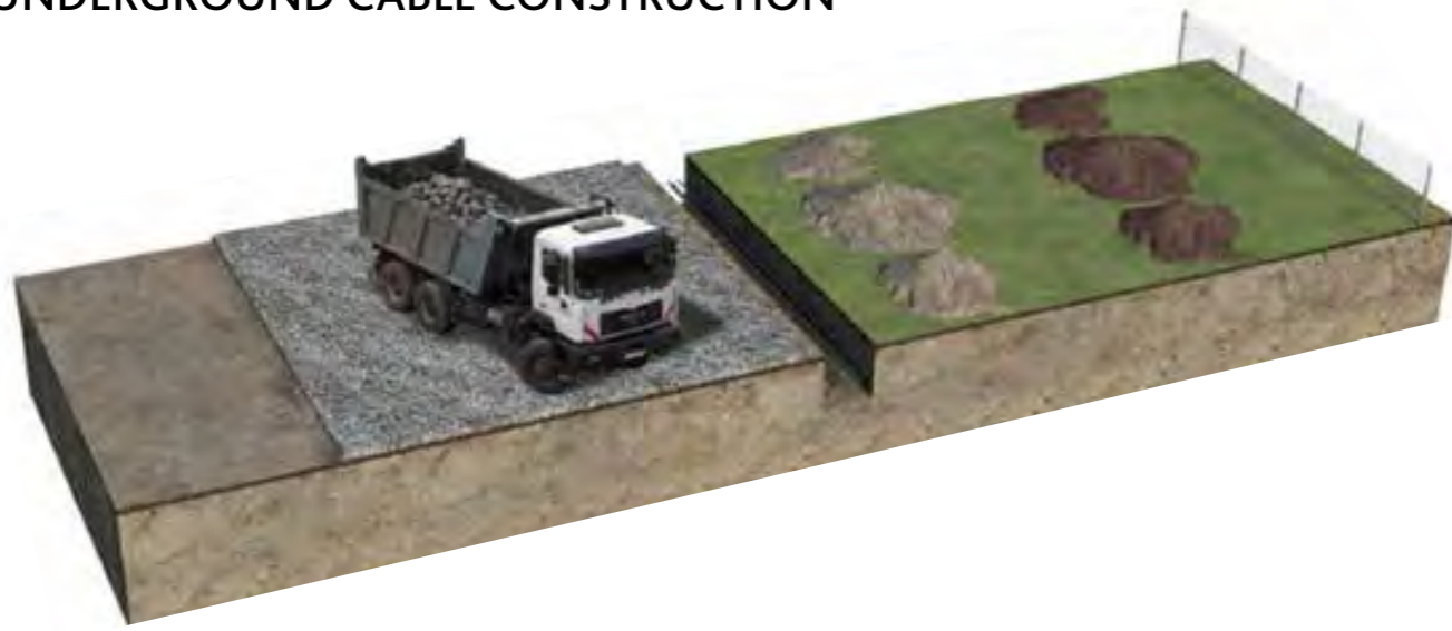
Figure 2 Construction of a 132kV line using underground cable
