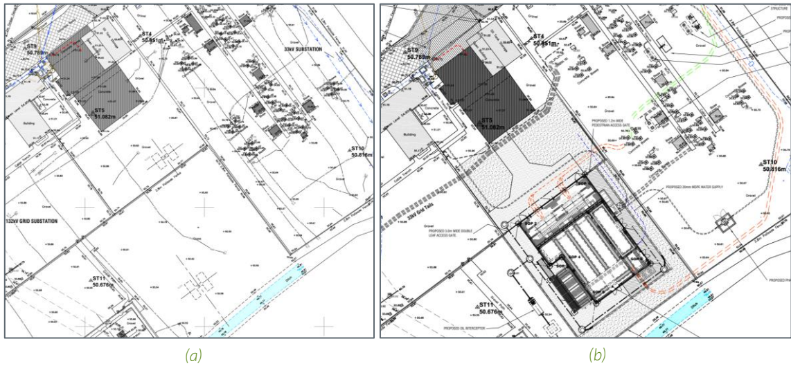
Figure 3-6 (a) Bangor Grid original site layout. (b) Bangor Grid existing site layout with MVDC converter building showing diverted cables.
