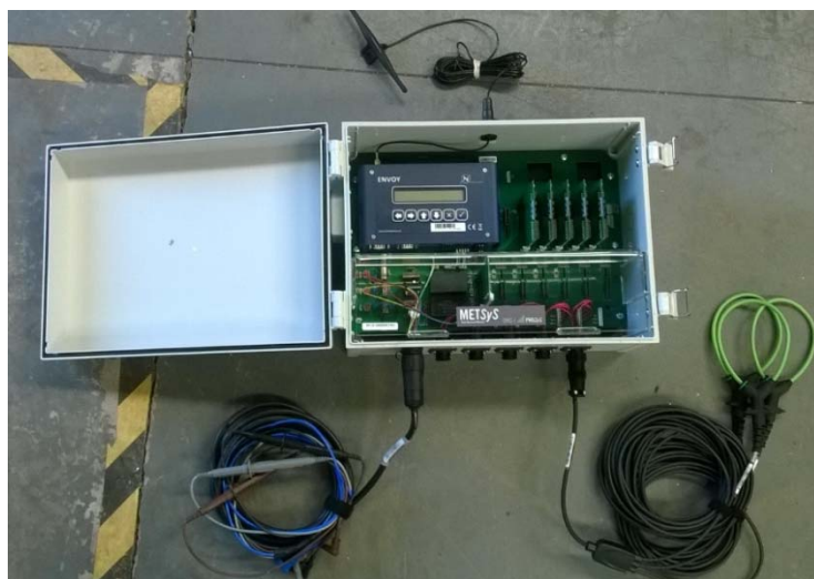
Figure 9: GMC-I METS y substation monitor
