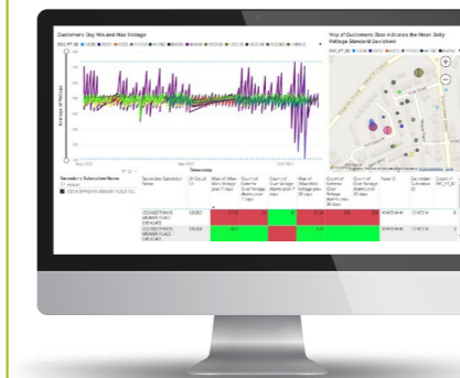
Smart meter voltage profiles used to identify faults on the network.
