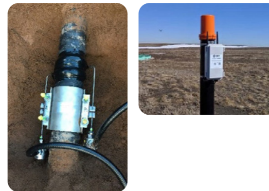
Figure 3. Sensor unit on cable (left) and communication of temperature data via RPMA wireless technology (right)
